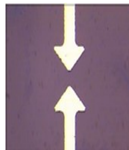
Fig.6. Top-view of one pair of electrode from microscope.
