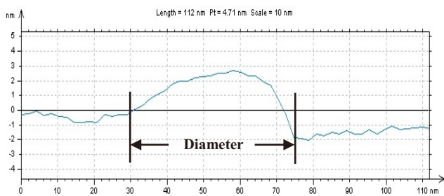
Fig.12. 112nm long cross-section line for CNT size measurement.
