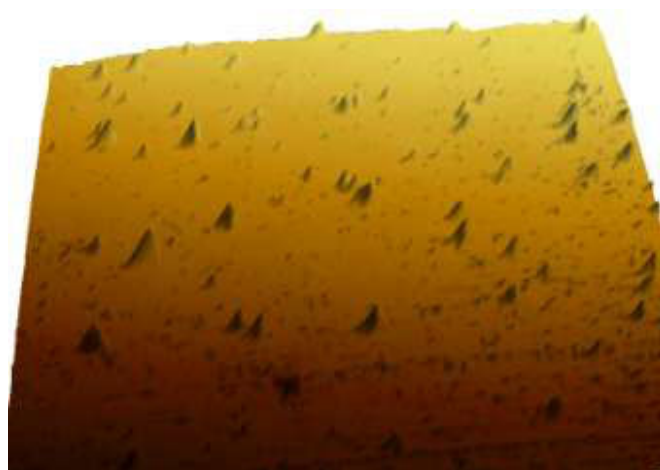
Fig. 7 3-D scan image of the acetic acid treated 2-D scan.
